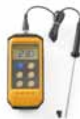
THERMOMETRE A SONDE RESISTANT AUX CHOCS -50°C/300°C
